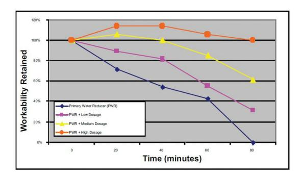
Do not use MasterGlenium SKY 909 admixture with admixtures containing beta-naphthalene sulfonate. Erratic behaviors in slump, workability retention and pumpability may be experienced.
